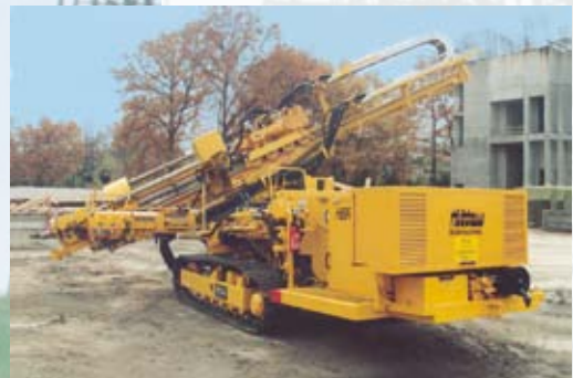
Mobile deep drill rigs, Hütte & Co.
